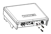
Loosen the swivel nut of the cable gland on the communication plate, remove the sealing plug and lead the stripped cable through the cable gland and communication plate, press the latch of the smart meter terminal and insert the stripped cable accordingly. Make sure the cable is connected firmly.
